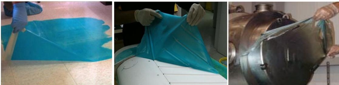
When dry, the product locks the contaminants into a polymer matrix. The film containing the encapsulated contamination can then be peeled. DeconGel peels from most non-porous and porous hard surfaces if the dried film is thick enough. If the film is difficult to peel, add another coat, let dry, and peel. In most cases the DeconGel will come off in a single sheet but for odd shaped surfaces you may be required to score DeconGel in order to peel it off.
