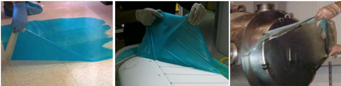
When dry, the product locks the contaminants into a polymer matrix. The film containing the encapsulated contamination can then be peeled. DeconGel peels from most non-porous and porous hard surfaces if the dried film is thick enough. If the film is difficult to peel, add another coat, let dry, and peel. In most cases the DeconGel will come off in a single sheet but for odd shaped surfaces you may be required to score DeconGel in order to peel it off.
