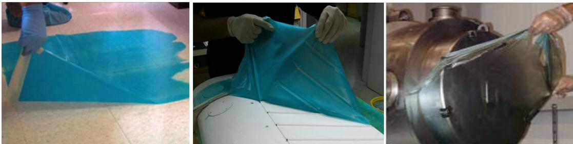
When dry, the product locks the contaminants into a polymer matrix. The film containing the encapsulated contamination can then be peeled. DeconGel peels from most non-porous and porous hard surfaces if the dried film is thick enough. If the film is difficult to peel, add another coat, let dry, and peel.
