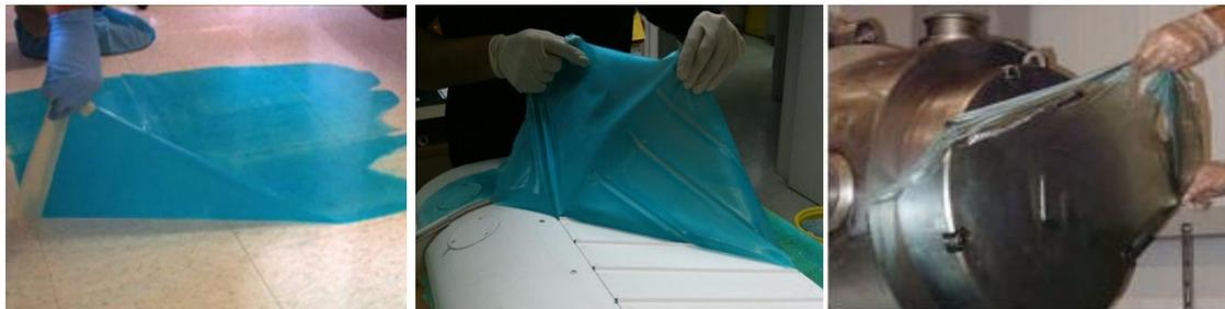
When dry, the product locks the contaminants into a polymer matrix. The film containing the encapsulated contamination can then be peeled. DeconGel peels from most non-porous and porous hard surfaces if the dried film is thick enough. If the film is difficult to peel, add another coat, let dry, and peel. In most cases the DeconGel will come off in a single sheet but for odd shaped surfaces you may be required to score DeconGel in order to be able to peel it off.
